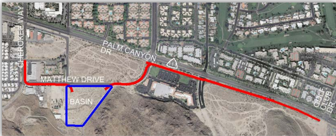
FIGURE 1: PALM SPRINGS MDP LINE 41, STAGE 3 - UNDERGROUND STORM DRAIN WITH DETENTION BASIN
